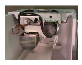
When the plate reaches the evaporator, the cam arm switch lever moves the actuator toggle switch to the right position. This stops the actuator motor and sets up the circuit to lower the plate in the next harvest cycle. It also energizes the pump motor and the board de-energizes the inlet water valve. The Freeze Cycle now begins.
